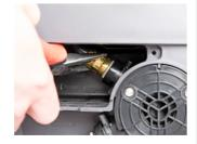
4.2 Using the pliers, remove the quick-connect clip.
