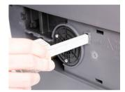
6.3 Begin retracting the new hose into the reel. Stop retracting with about 50cm of hose out of the reel.
